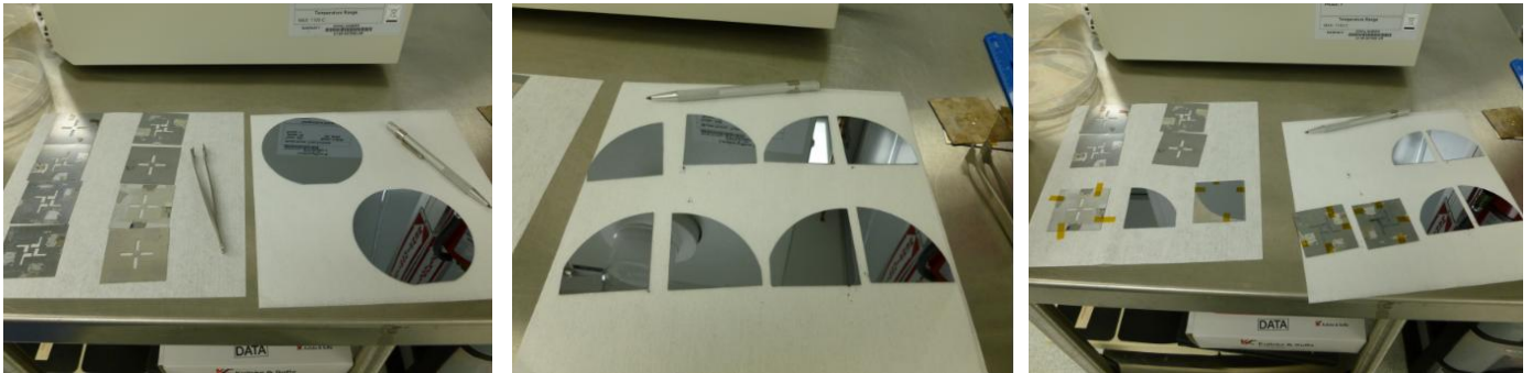
Figure V: Shadow masks and 3" wafers used for this study (left) cleaved samples (center) and cleaved samples being mounted to shadow masks (right)
