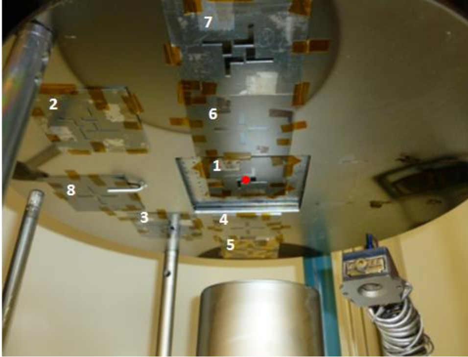
Figure VI: Locations and identities of the 8 shadowed samples which were mounted at varying distances, \ell_2 through \ell_8 , from the point source in the evaporator. The red dot in the center of the figure represents the location directly above the point source (sample 1).
